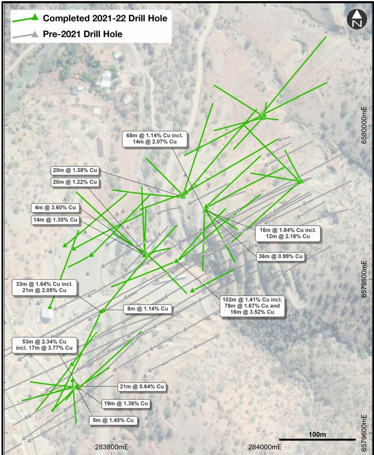
Figure 3: Dalmacia North Target Drill Collar Plan
