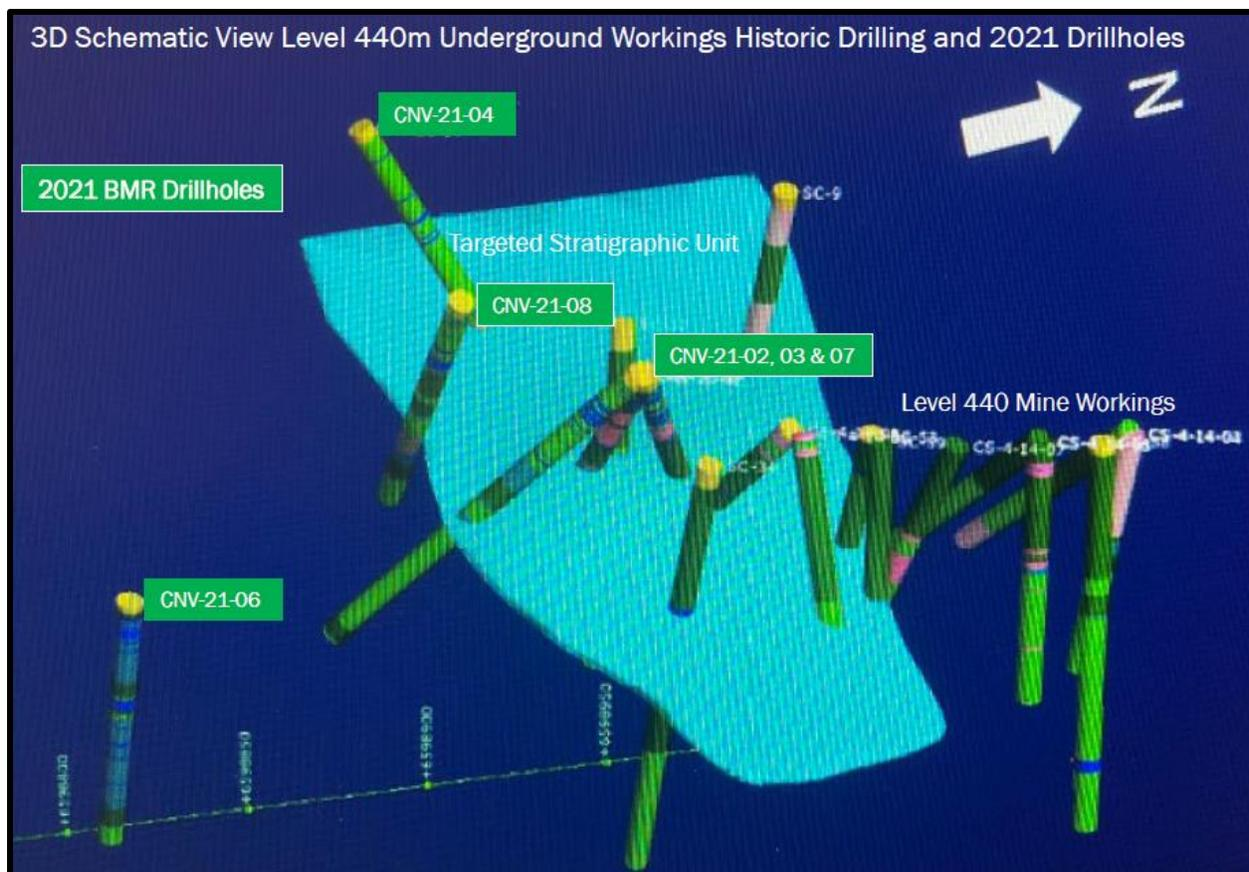
Figure 8: Cinabrio South Target 3D Schematic View Level 440m Workings & Drilling
