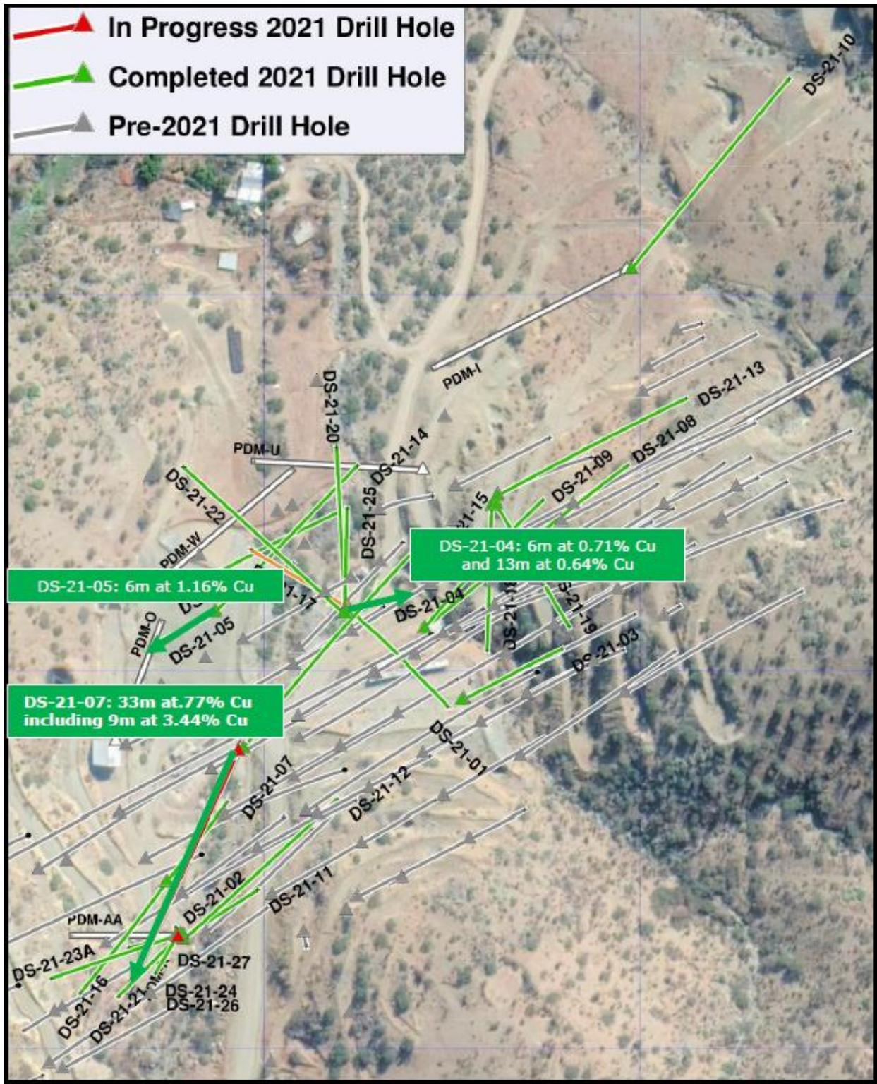
Figure 2: Dalmacia Target Drill Collar Plan with Recent Copper Intercepts
