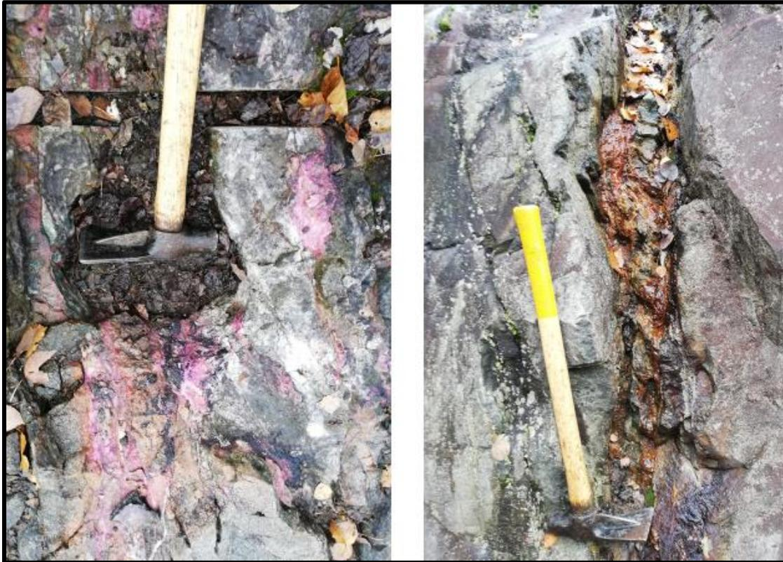
Photo 1: Left-typical Calcite (+/-quartz) vein with Cobalt bloom; Right- typical specular hematite vein; both types are found on the Bald Rock outcrop and in the historic prospect cut/pit.
