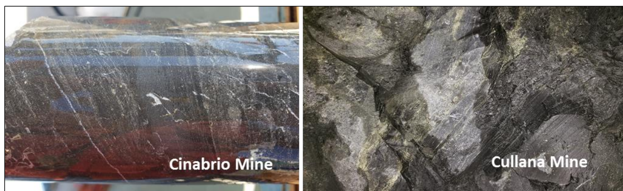
Figure 7-12: Typical Sulphide Copper Mineralization from Cinabrio Mine and Near-by Cullana Operation
