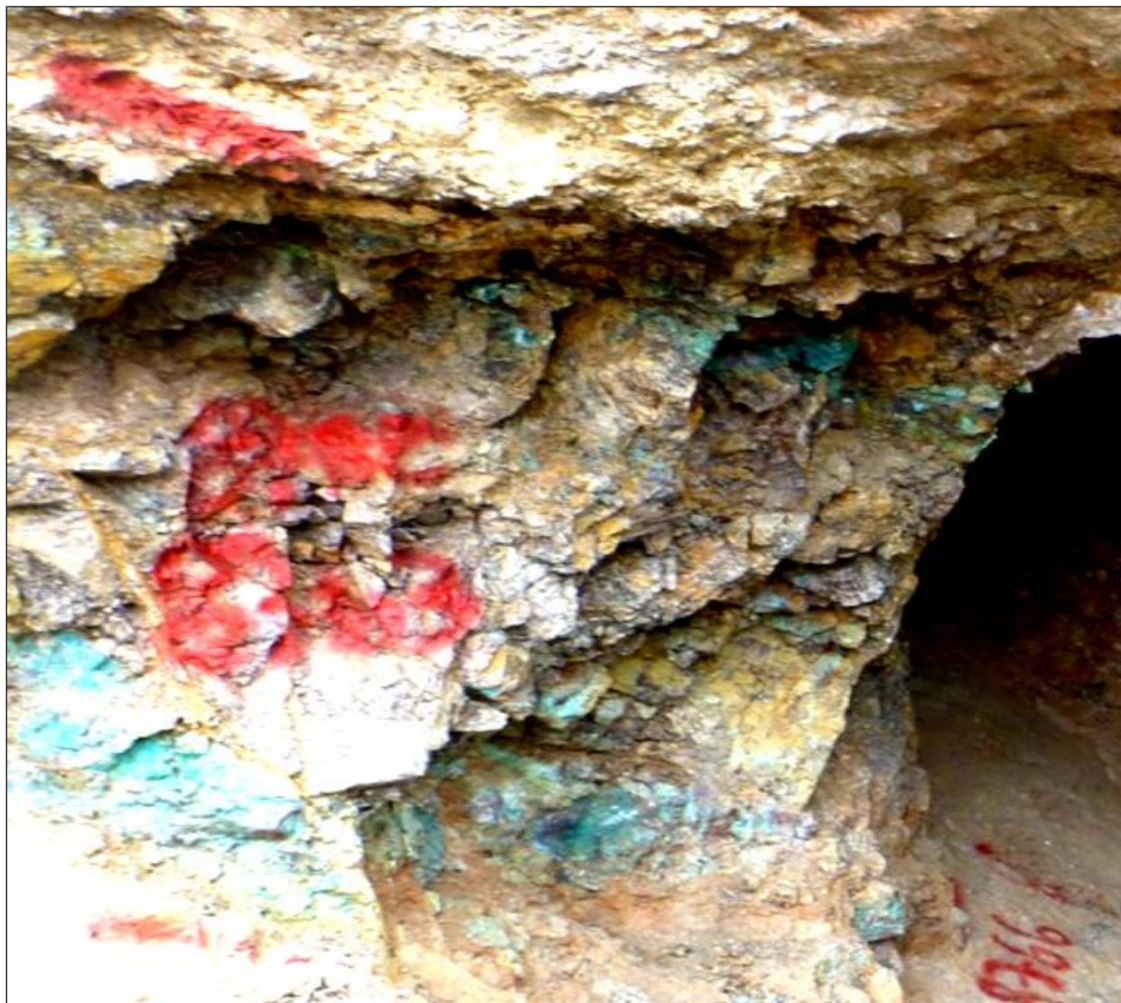
Figure 9-9: Structurally Controlled Copper Oxide Mineralization - Wall of Historic Working
