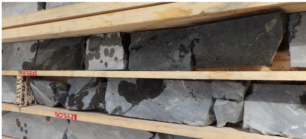
Figure 10-10: Typical Sawn Core Sample
