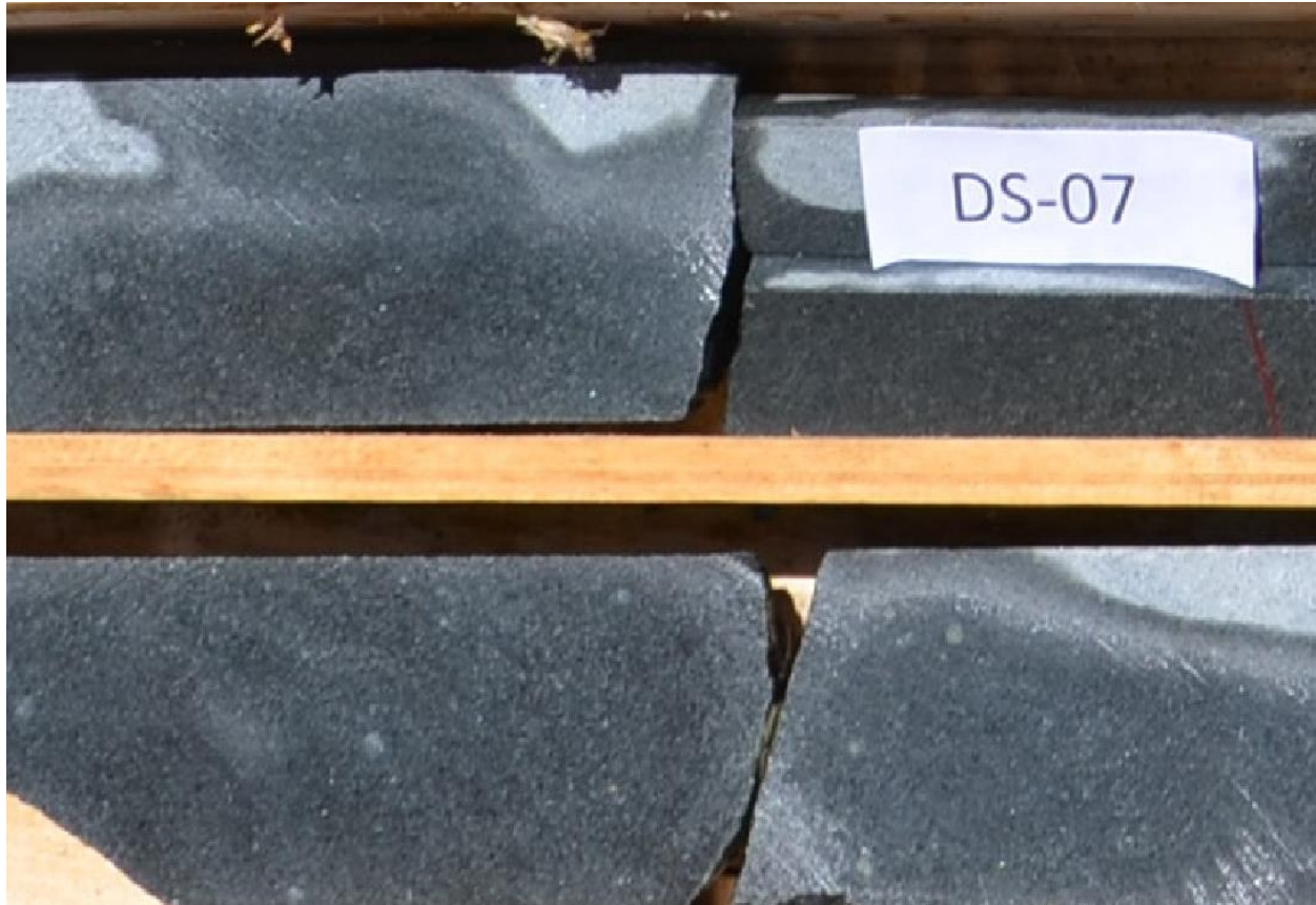
Figure 7-34: Ocoite with Secondary Biotite
