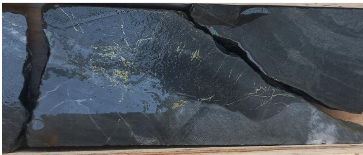
Figure 7-18: Cinabrio Fracture Controlled Chalcopryrite- Pyrite Mineralization in TSU Shale Unit
