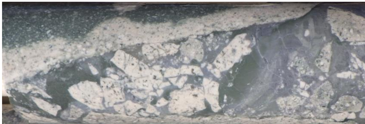
Figure 7-47: Auto-Brecciated Andesite Lava Flow in Drill Hole CNN-22-40 308 m
