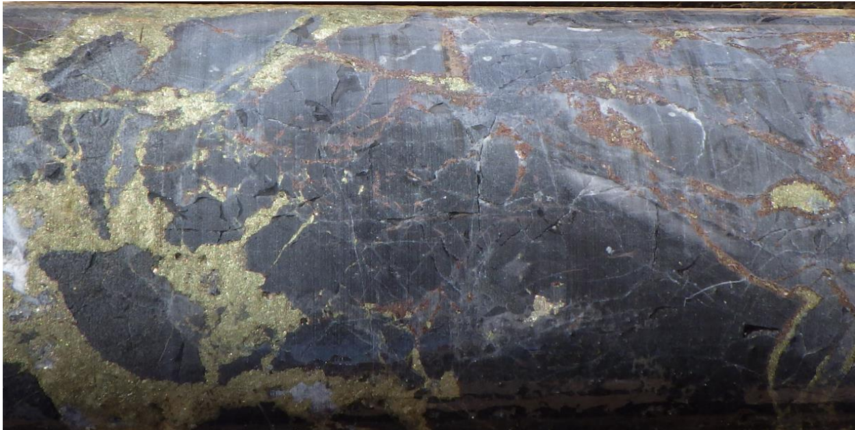
Figure 7-54: Chalcopyrite and Sphalerite Veinlets and Breccia Infill from Drill Hole CNN-21-30: 268 m
