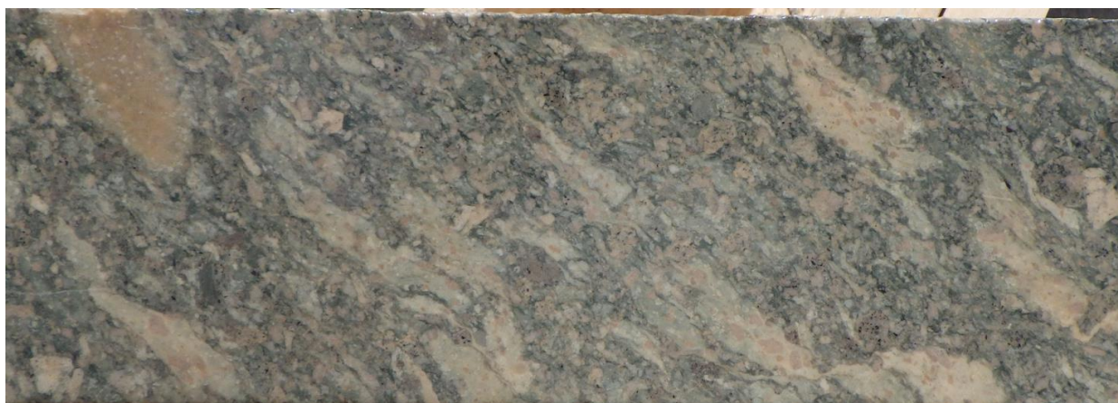
Figure 7-22: Ignimbrite Tuff: Drill Hole: SAS-21-08: 232 m
