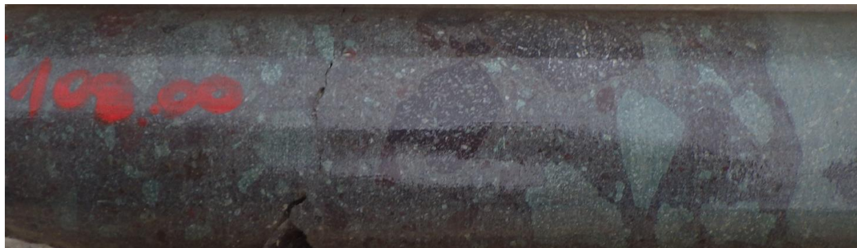
Figure 7-23: Volcanic Breccia: Drill Hole: SAS-21-06: 108 m
