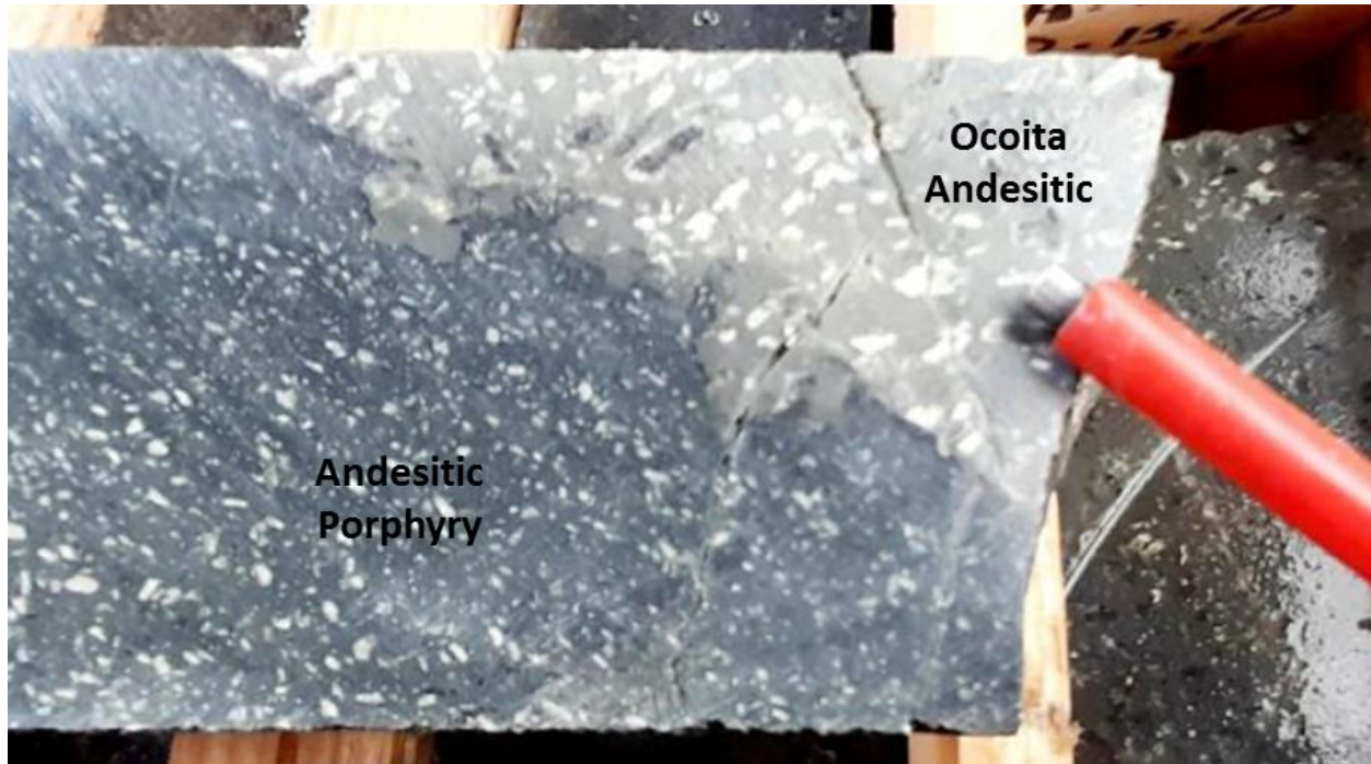
Figure 7-36: Andesite Porphyry Cutting Ocoite
