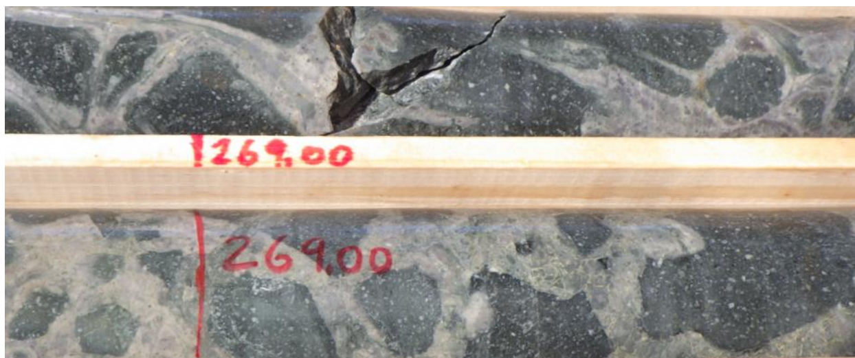
Figure 7-48: Auto-Brecciated Andesite Lava Flow in Drill Hole CNN-22-39: 269 m
