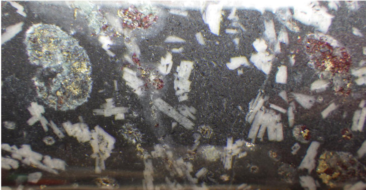
Figure 7-42: Bornite - Chalcopyrite Infill and Veinlets with Quartz, Chlorite and Sericite in Vesicular Ocoite
