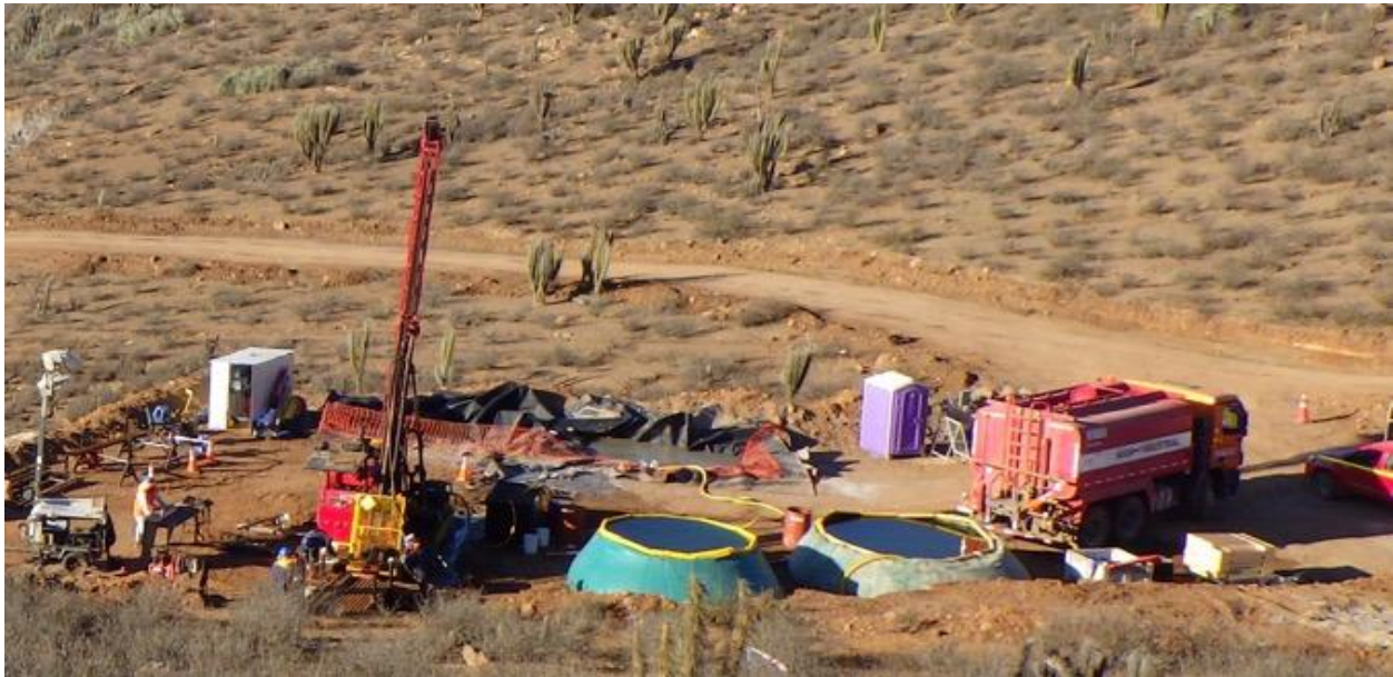
Figure 10-15: San Andres Drilling 2021 – Close-up View Diamond Drill Rig in Operation
