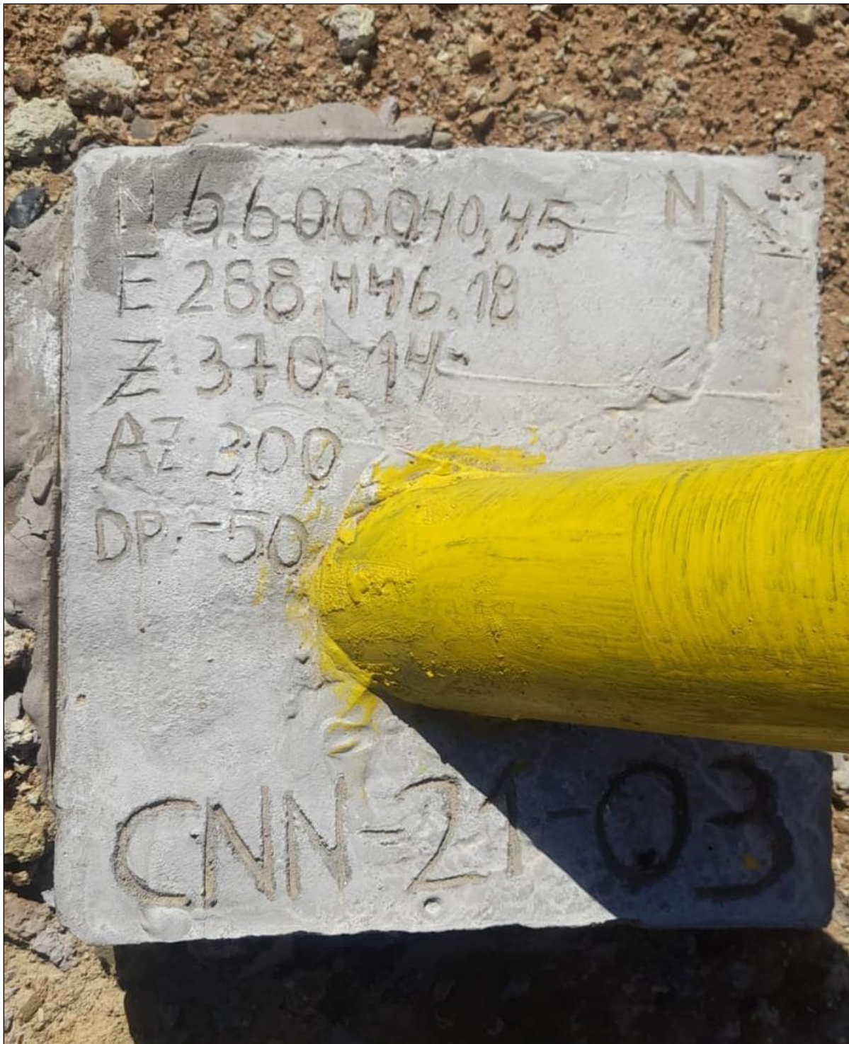
Figure 10-5: Close-up View of Typical Drill Collar Marker – Cinabrio Norte
