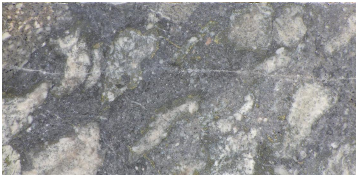
Figure 7-27: Disseminated Chalcopyrite and Aggregates Around Clasts in Tuff Breccia in Drill Hole SAS-21-08: 226 m
