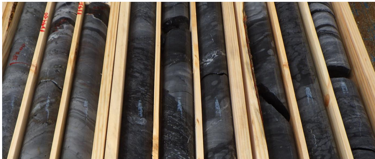
Figure 7-45: Laminated Shales Sequence in Drill Hole CNN-22-41: 393 m – 400 m
